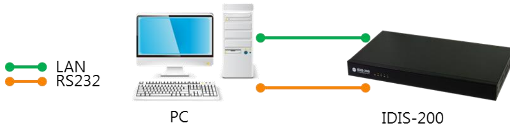
Figure 2-1 Connection for configuration
