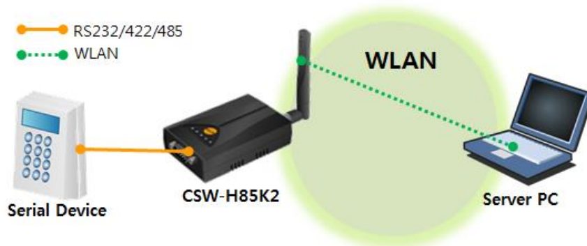
Figure 1-1 1:1 network with a PC
