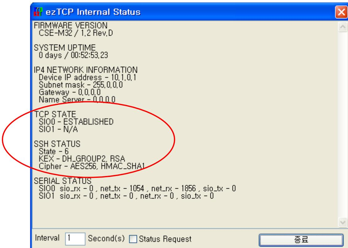
User can confirm "TCP STATE" / "SIO0 – ESTABLISHED" and "SSH STATUS" / "State – 6", "Cipher – AES\_256, HMAC\_SHA1".
