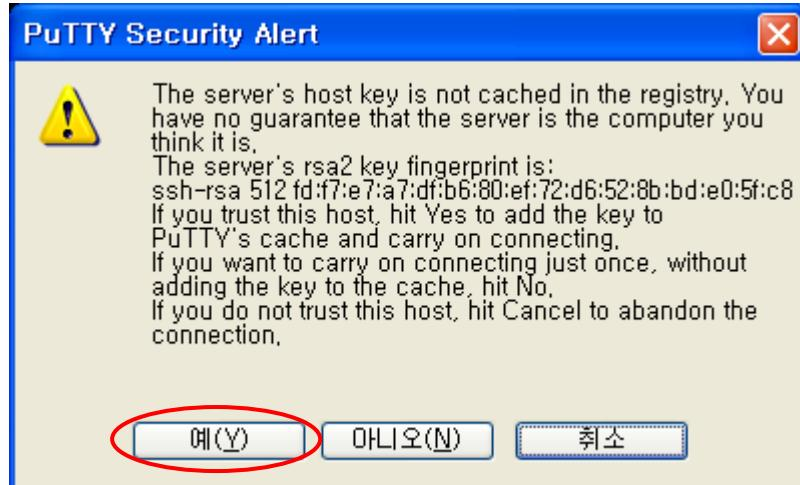
When and if the SSH server's key is not cached in SSH client, the SSH client ask whether it save the server's key. After saving the server's key once, the SSH client doesn't ask it again. If user change the key of ezTCP the SSH client will ask it again.
